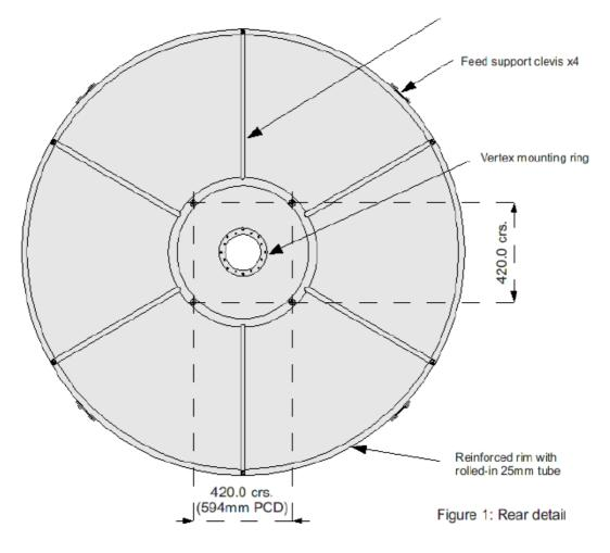
This high grade reflector antenna assembly features adjustable subreflector support arms, rugged construction and a durable finish. It is supplied flat packed for economical transport and can be assembled quickly on site.
