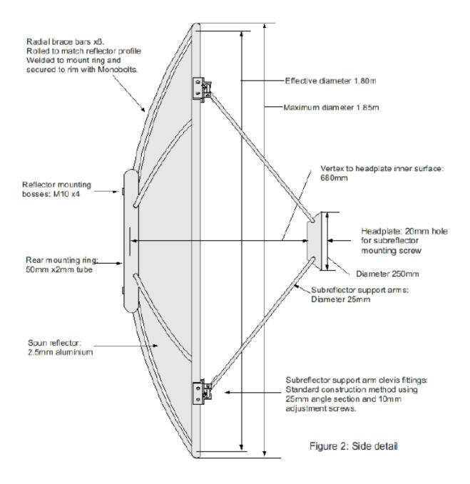
The reflector spinning is stabilised and protected against high wind loadings by six radial brace bars fixed between the outer rim and the mount ring. The feed is secured to the reflector by a precision machined vertex mount.
