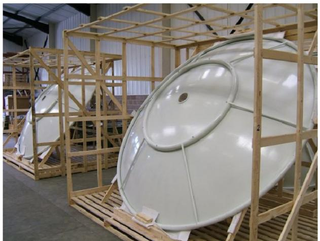
**Elite Antennas** manufacture spun, prime-focus aluminium reflectors for commercial, military and research applications. We offer a range of reflector assemblies in popular sizes, as well as the capacity to tailor reflectors to the requirements of our customers. Our flexible build system allows prototyping and one-off work to be completed rapidly and economically, while allowing straightforward integration or subsequent engineering operations. other benefits of spun reflectors include:
